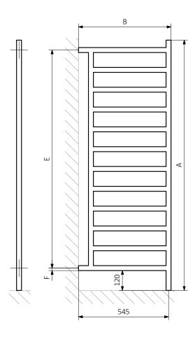
A — Height B — Width C1-C5 — Distance between pipe centres D — Horizontal distance between mounting bracket centres E — Vertical distance between mounting brackets F — Distance between a mounting bracket and the bottom of the radiator
