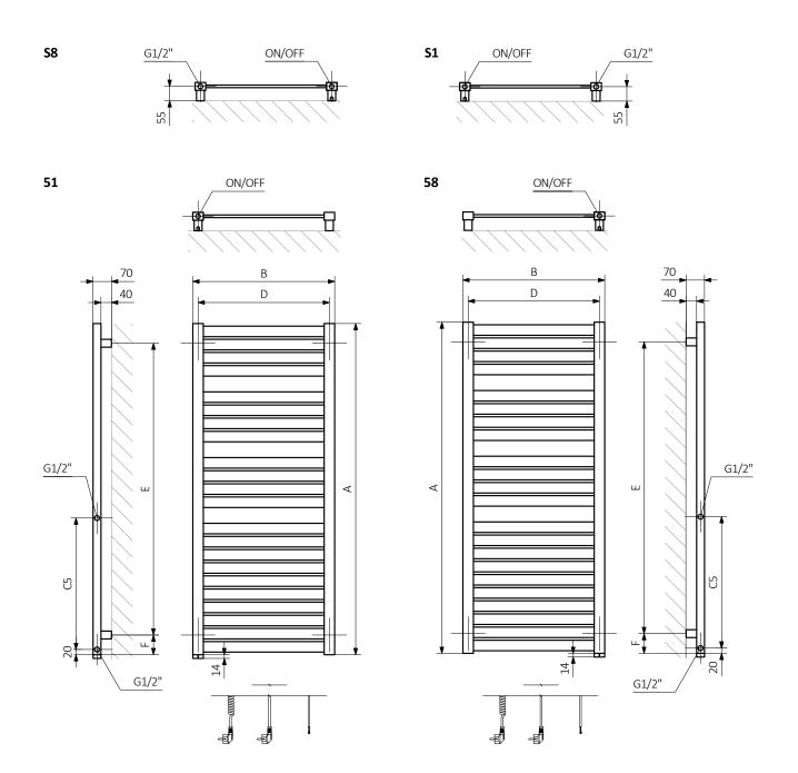
A - Height B - Width C1-C5 - Distance between pipe centres D - Horizontal distance between mounting bracket centres E - Vertical distance between mounting brackets F - Distance between a mounting bracket and the bottom of the radiator
